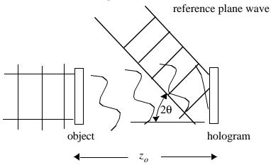
The reference beam is tilted. This is a real "hero" experiment without a laser. Holography was made practical after the invention of the laser.
