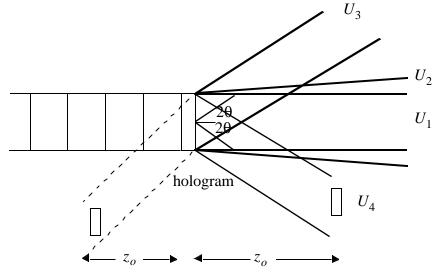
The reconstruction beam is a plane wave at normal incidence, with amplitude B.
