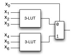
This type of structure is common in FPGAs to easily allow two N-LUTs to be combined to form a (N+1)-LUT. You are asked to implement a *4-input Multiplexor* circuit using this FPGA. How many of the above combinational logic blocks would be needed? Show your implementation.
