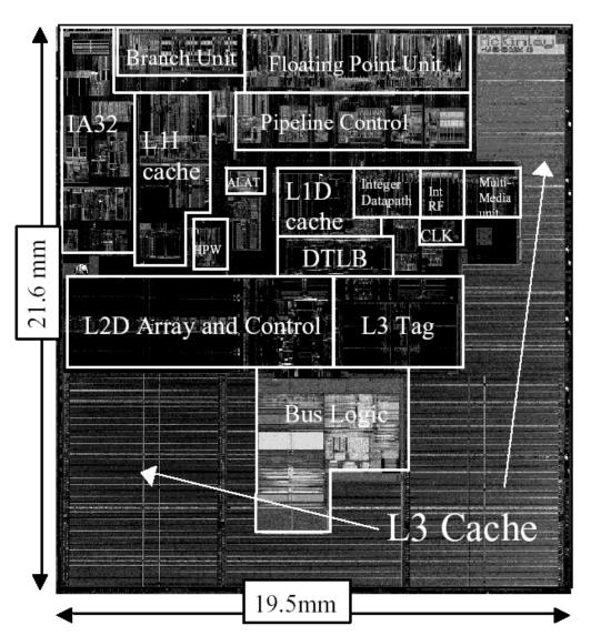
Level 1: 16KB, 4-way s.a., 64B line, quad-port (2 load+2 store), single cycle latency
