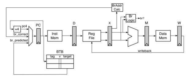
The BTB has been added in the Fetch Stage. The BTB is indexed by the PC register in the Fetch Stage. Branch address calculation has been moved back to the Execute Stage.
