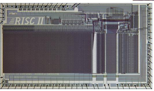
RISC-II (1983) contains 40,760 transistors, was fabbed in 3  $\mu$ m NMOS, ran at 3 MHz, and the size is 60 mm<sup>2</sup>.
