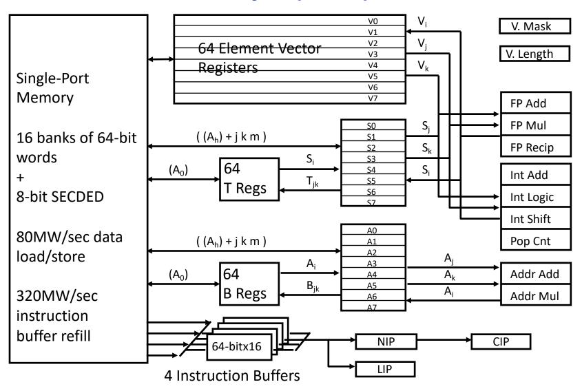
memory bank cycle 50 ns processor cycle 12.5 ns (80MHz)
