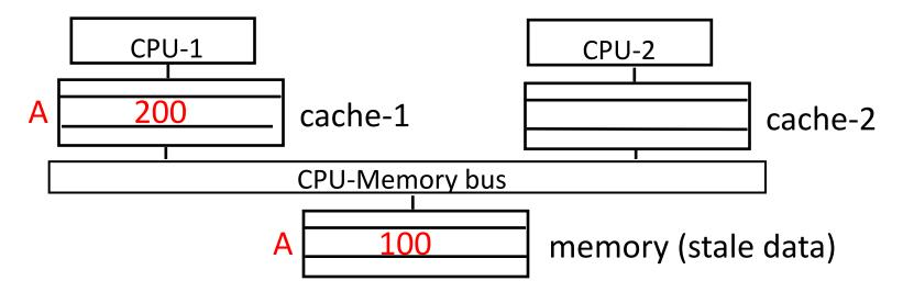
When a read-miss for A occurs in cache-2, a read request for A is placed on the bus
