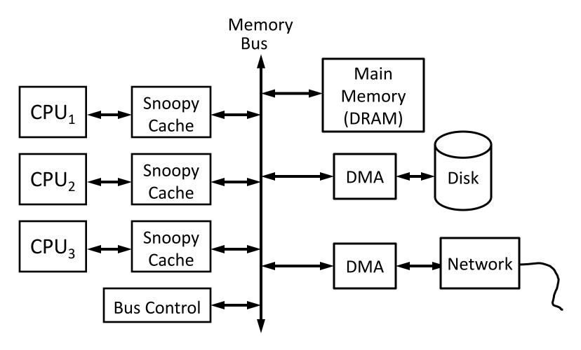
Use snoopy mechanism to keep all processors' view of memory coherent
