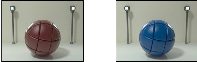
BRDFs for aerosol spray paint
