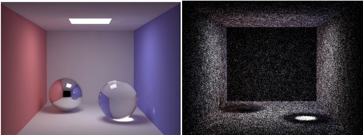
Figure 8: The image on the left is a Cornell Box rendering using 200,000 global photons and 50,000 caustic photons. The image on the right is the photon map.
