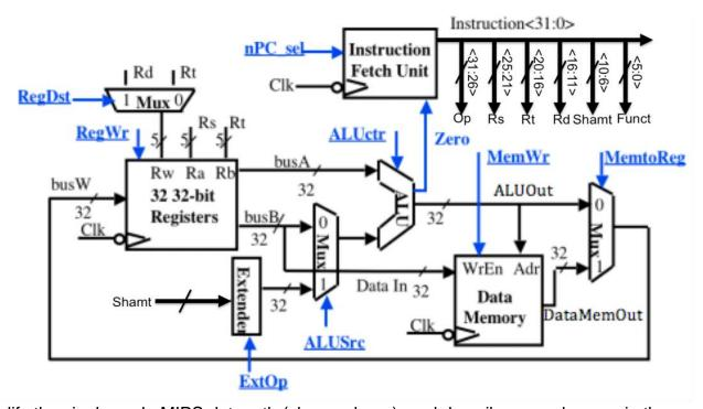
a) Modify the single-cycle MIPS datapath (shown above), and describe your changes in the space below. Your modification may use simple adders, mux chips, wires, and new control signals. You may replace original labels where necessary.
