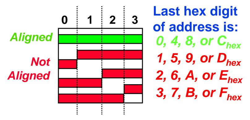
• Called Alignment: objects must fall on address that is multiple of their size.
