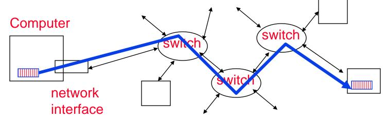
ability to name the components and to route packets of information messages - from a source to a destination
