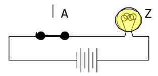
close switch (if A is "1" or asserted) and turn on light bulb (Z)
