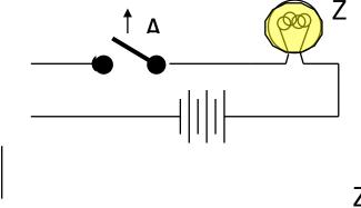
open switch (if A is "O" or unasserted) and turn off light bulb (Z)
