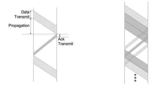
Figure 1: Stop-and-Wait Figure 2: Sliding Window with SWS=RWS=3
