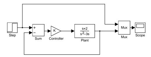
Now, replace the variable "K" with a "1" in the constant gain controller. Run the simulation and see what happens. Is the output stable? Increase the gain to 2 and re-run the simulation. Continue increasing the gain to 10, and observe the results.
