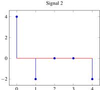
Assume that both signals are periodic with period 5, that is, each plot shows one full period of a periodic signal.
