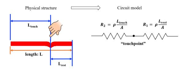
We then connect a voltage source  $V_s$  to the two ends of the circuit model we just built.
