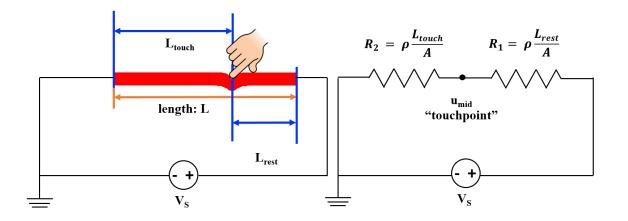
Actually, we have already analyzed this circuit model we just built at the beginning of the note, this is just a voltage divider circuit! First we know that,
