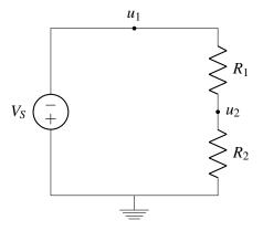
• Step 3: Label the current through every non-wire element in the circuit with  $i_n$ .
