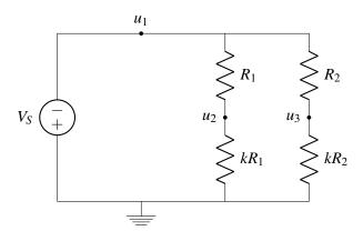
Given the knowledge we have for the voltage divider circuit, we actually do not have to apply the circuit analysis algorithm to this interesting circuit to derive  $u_1$ ,  $u_2$ ,  $u_3$ .
