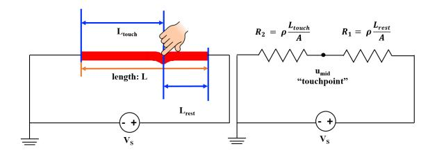
By using a voltage divider circuit, we can map  $u_{mid}$  to  $L_{touch}$ . A relationship between  $u_{mid}$  and  $L_{touch}$  exists such that:
