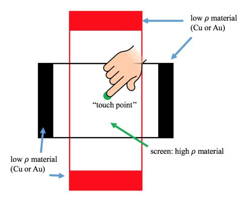
The left and right ends of the top red plate as well as the left and right ends of the bottom black plate are made of materials that have very low resistivities  $\rho$ , we can treat them as ideal wires ( $\rho = 0$ ). The materials of the transparent screen that we touch in the middle have much higher resistivity.
