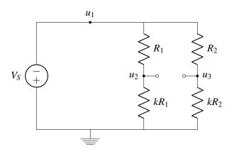
Now, the interesting circuit becomes the same as before the addition of  $R_3$ . Our bold assumption that  $R_3$  will not affect circuit operation is indeed correct. By replacing  $R_3$  with an open circuit after fguring out  $R_3$  is at (0, 0) on the I-V plot, we can write down  $u_2, u_3$  directly:
