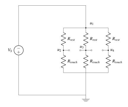
After replacing horizontal resistors with open circuit, we can use a voltmeter and measure  $u_3$ , which is:
