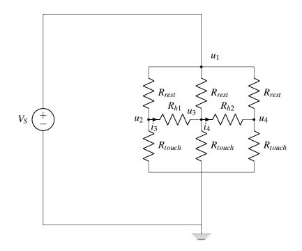
Since  $R_{rest}$  and  $R_{touch}$  are the same for each segment, we can replace horizontal resistors  $R_{h1}$ ,  $R_{h2}$  like we did when analyzing the interesting circuit because  $u_2 = u_3$ ,  $u_3 = u_4$ .
