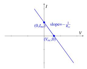
An interesting note is that we can move back and forth between Thevenin and Norton equivalent representations using their relationship through Ohm's Law. Because  $V_{Th}$  and  $I_N$  represent two points on the same line, we know that  $I_{sc} = \frac{V_{Th}}{R_{th}}$  by Ohm's law. Hence, we can find both equivalent circuits by solving for just one. Conversely, we cn solve for both  $V_{Th}$  and  $I_N$  and then find  $R_{Th}$  by computing  $R_{Th} = \frac{V_{Th}}{I_N}$ .
