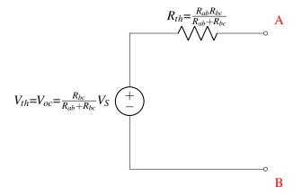
If we instead chose the upper two nodes (instead of the lower two nodes) as the two terminals (nodes A and B) as follows for the same exact circuit and find an equivalent Thevenin circuit from the standpoint of these two nodes,
