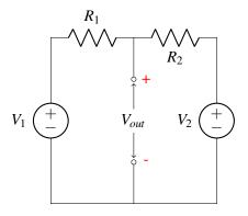
The procedure to do this (which is known as superposition) is as follows: **For each source** *k* (either voltage source or current source)
