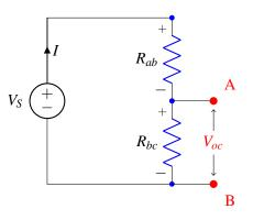
Note that the same current flows through the two resistors and that  $V_{Rab} = V_s - V_{oc}$ . Therefore, using Ohm's Law:
