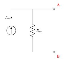
What about solving for the Norton equivalent circuit? It is important to note that  $R_N$  is equal to  $R_{Th}$ , meaning the slope of the IV curve is the same. Now, instead of looking at the V axis intercept, we find the intersection with the *I*-axis: At this point, the voltage across A and B is equal to zero, which is equivalent to shorting A and B. We denote the current at this point be  $I_{SC}$ .
