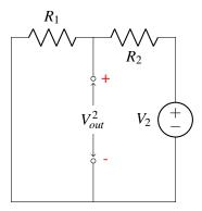
We again recognize that this is just a voltage divider circuit and therefore we can see that  $V_{out}^2 = \frac{R_1}{R_1 + R_2}V_2$ . Finally, to get the output voltage  $V_{out}$  of the original circuit, we add the two output voltages based on the response of each voltage source together  $V_{out} = V_{out}^1 + V_{out}^2 = \frac{R_2}{R_1 + R_2}V_1 + \frac{R_1}{R_1 + R_2}V_2$ .
