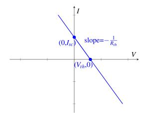
We call the first circuit below, containing a voltage source and a resistor the **Thevenin equivalent circuit**; we call the second circuit, containing a current source and a resistor, the **Norton equivalent circuit**. Once we simplify the original circuit to one of the above, we can easily figure out  $V_{out}$  no matter what resistor it is connected to on the right. In fact, we can convert **any** circuit into any one of the equivalent forms above.
