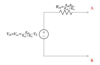
This is not the same result! This simple example shows how picking two different nodes in the same circuit and finding equivalent circuits will produce a different results. (And more generally, all circuits may or may not behave in the same from the standpoint of any two nodes) This is an important distinction to be made when looking at equivalent circuits. We are simply finding an equivalent circuit from the standpoint of a pair of terminals.
