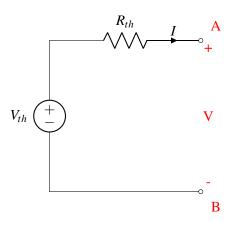
Now how would you figure out  $V_{th}$  and  $R_{th}$  for the Thevenin equivalent circuit?
