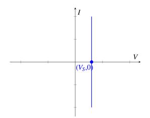
Now if we want to zero out this voltage source, we are setting  $V_S = 0$ . Then the I-V plot is exactly the y-axis.
