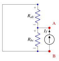
We can see that this is the same as the parallel resistor case we examined above: therefore,  $R_{Th} = \frac{V_T}{I_T} = R_{ab} \parallel R_{bc}$ .
