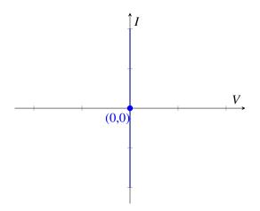
What does this mean? This means that it allows any current to go through, however the voltage drop always remains zero. This is exactly what a short circuit does.
