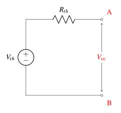
**Step 2, find**  $R_{Th}$ : Zero out any independent sources. Remember, this means voltage sources turn into a wire and current sources turn into an open circuit. Then apply either a test current into the terminal and measure the resultant voltage, or apply a test voltage and measure the resultant current.  $R_{Th} = \frac{V_{test}}{I_{test}}$
