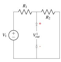
We can recognize this as just a voltage divider circuit, and therefore we know that  $V_{out}^1 = \frac{R_2}{R_1 + R_2} V_1$ . Next we compute the output voltage due to  $V_2$  and hence source  $V_1$  will be replaced with a wire.
