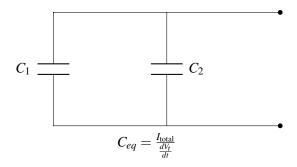
What is the equivalent capacitance? By analogy with our resistor case, we will try and apply a test voltage to this circuit:
