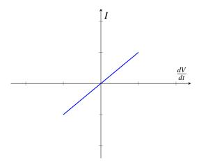
An important implication of this is in order for current to flow through the capacitor, the voltage across that capacitor must be changing with time. If the voltage is no longer increasing, then the current through the capacitor will equal 0.
