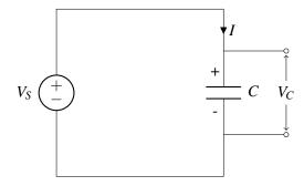
We know that initially, charges are going to build up on the two plates — positive charges on the top plate and negative charges on the bottom plate. Once enough charge has been stored, the voltage across the capacitor becomes  $V_C = V_S$ ; because the voltage can no longer increase past this point, the current I flowing through the circuit becomes zero.
