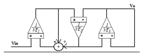
The diagram above, shows the integrator implementation of a 3<sup>rd</sup> order lowpass filter with a corner frequency of 18KHz and sampling frequency of 3.6MHz.
