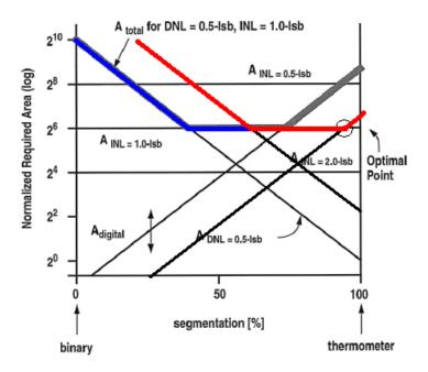
No, a more stringent DNL requirement would not affect the choice of segmentation since it is only the INL and digital circuitry area requirements that set the optimal point. If the DNL were required to be even more stringent such that the area required supercedes the INL requirement (at perhaps 1/16 LSB) then there would be a new optimal segmentation point.
