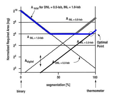
From the new curve, the optimal segmentation point is closer to 100%. This makes intuitive sense, since the limiting factor on moving to an entirely thermometer-coded approach is the overhead area of the digital decoding circuitry.
