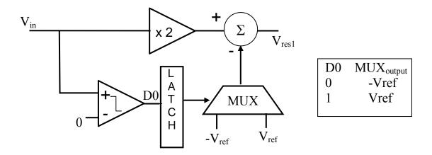
The rest of the stages have the block diagram shown bellow:
