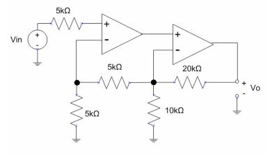
Since no current flows into the (+,1) terminal:  $V_{+,1} = V_{in}$
