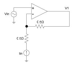
By the summing point constraint:  $V_{-} = V_{+} = V_{in}$ By Ohm's Law:  $V_{1} = V_{in} - I_{in}(0.5\Omega)$
