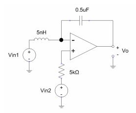
Since no current flows into the (+) terminal:  $V_{+} = V_{in2}$ By the summing point constraint:  $V_{-} = V_{in2}$ By KCL:  $V_{0} = V_{in2} - \frac{Z_{C}}{Z_{L}} (V_{in1} - V_{in2}), Z_{C} = \frac{1}{j\omega 0.5\mu F}, Z_{L} = j\omega 5nH$   $V_{0} = V_{in2} + \frac{1}{\omega^{2} (0.5\mu F)(5nH)} (V_{in1} - V_{in2})$
