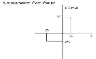
d) (7 pts) Plot electric field E(x) vs. distance x. Assuming the  $\epsilon$  is the permittivity of the material Label your plot. Write  $E_{max}$  as a function of  $x_N$ .
