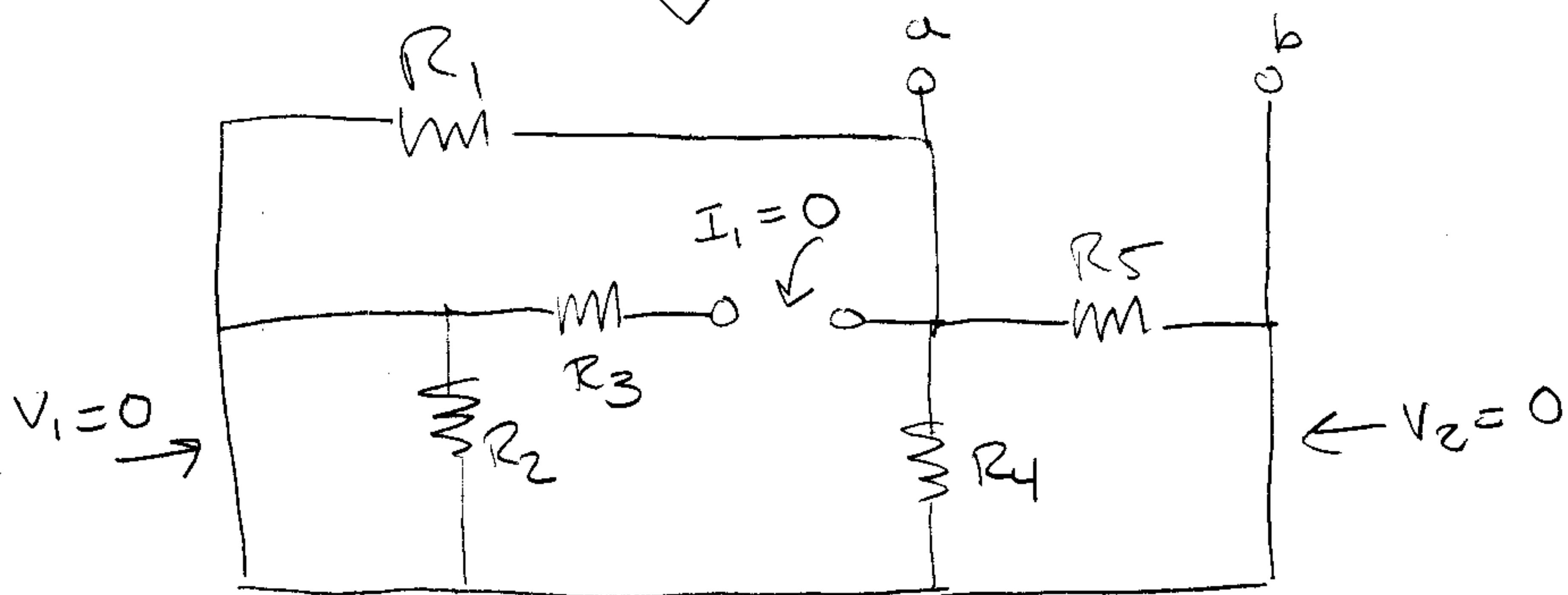
$R_2$  is in parallel with a wire ( $0\Omega$ ).
