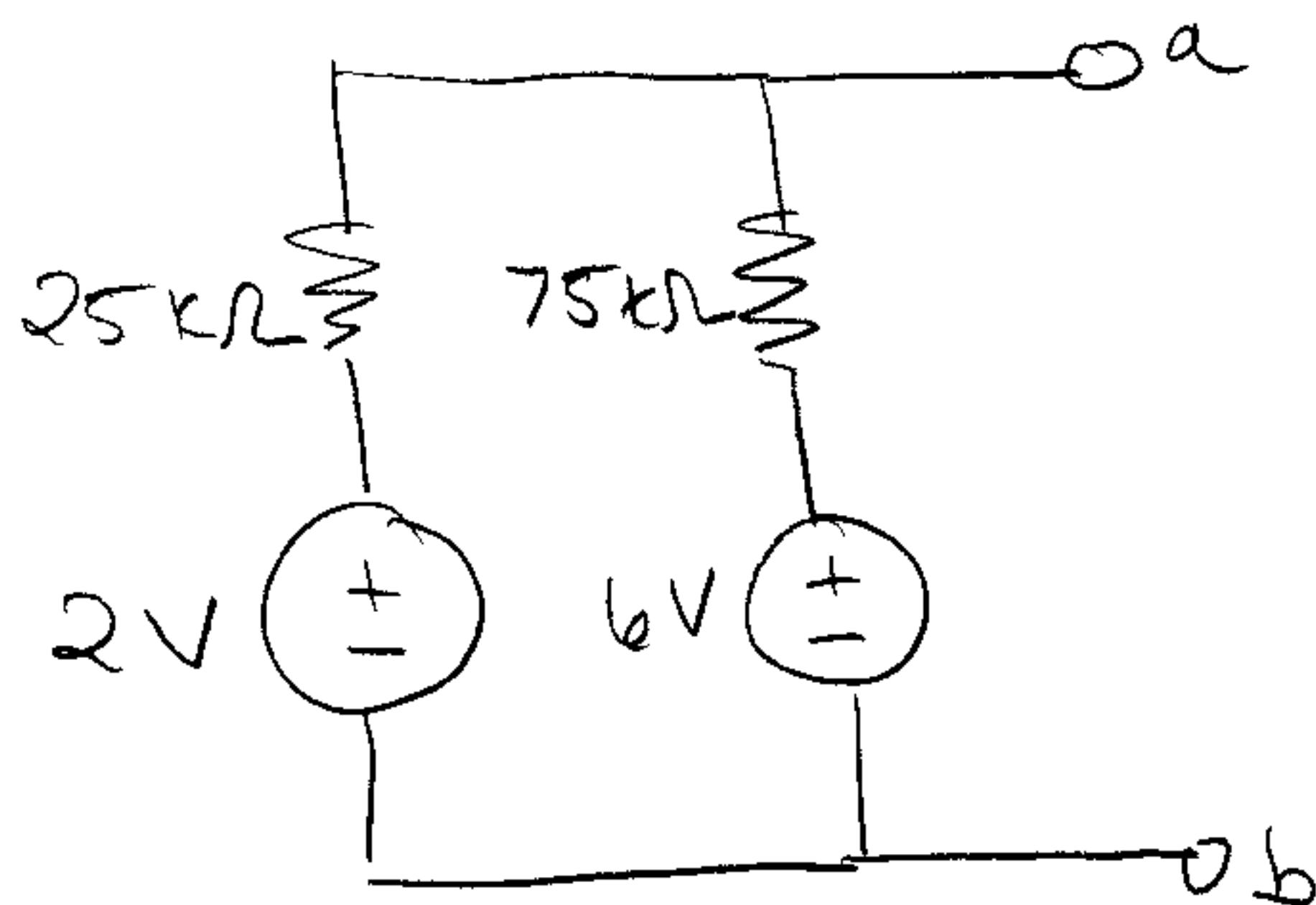
$$V_T = V_{ab} \text{ when } a-b \text{ open}$$
