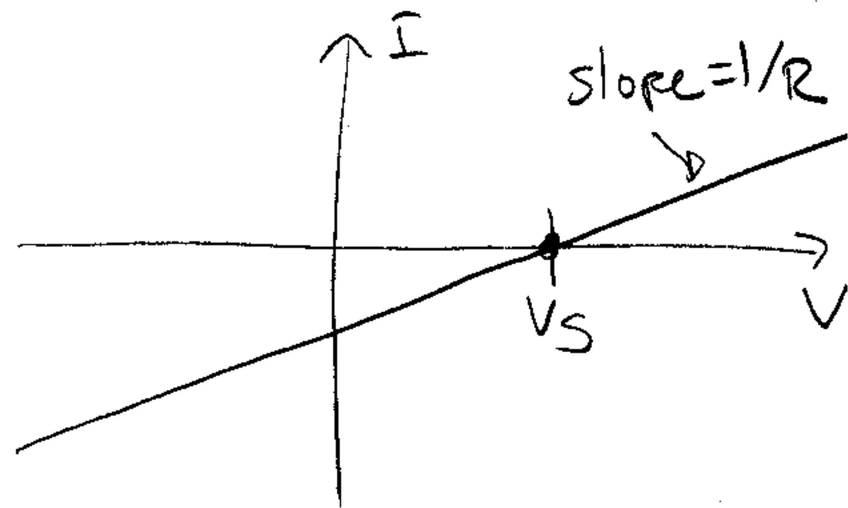
We can replicate any\* linear I-V characteristic graph through choice of  $V_s$  and  $R$ .
