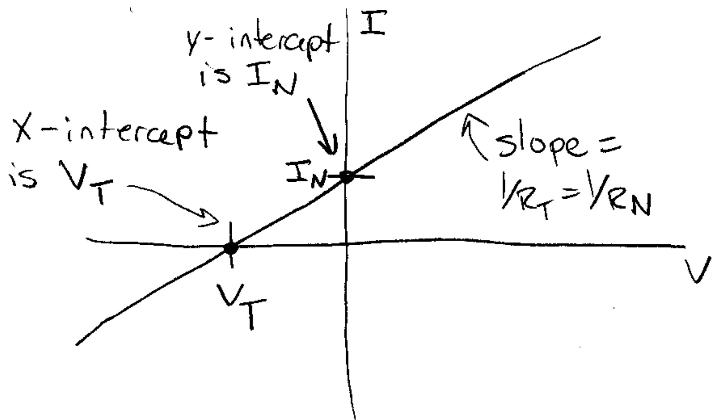
$$V_T = V_{ab} \text{ when } a-b \text{ open}$$
