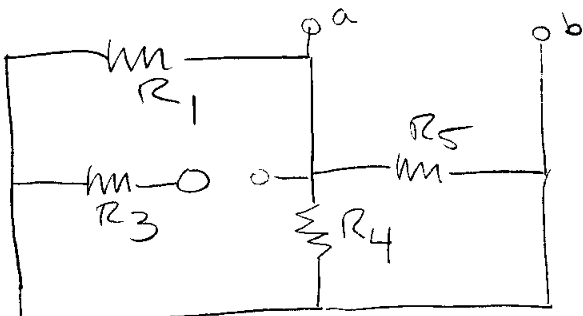
We want to find out how this network of resistors affects a device connected to a+b, i.e., the I-V characteristic.
