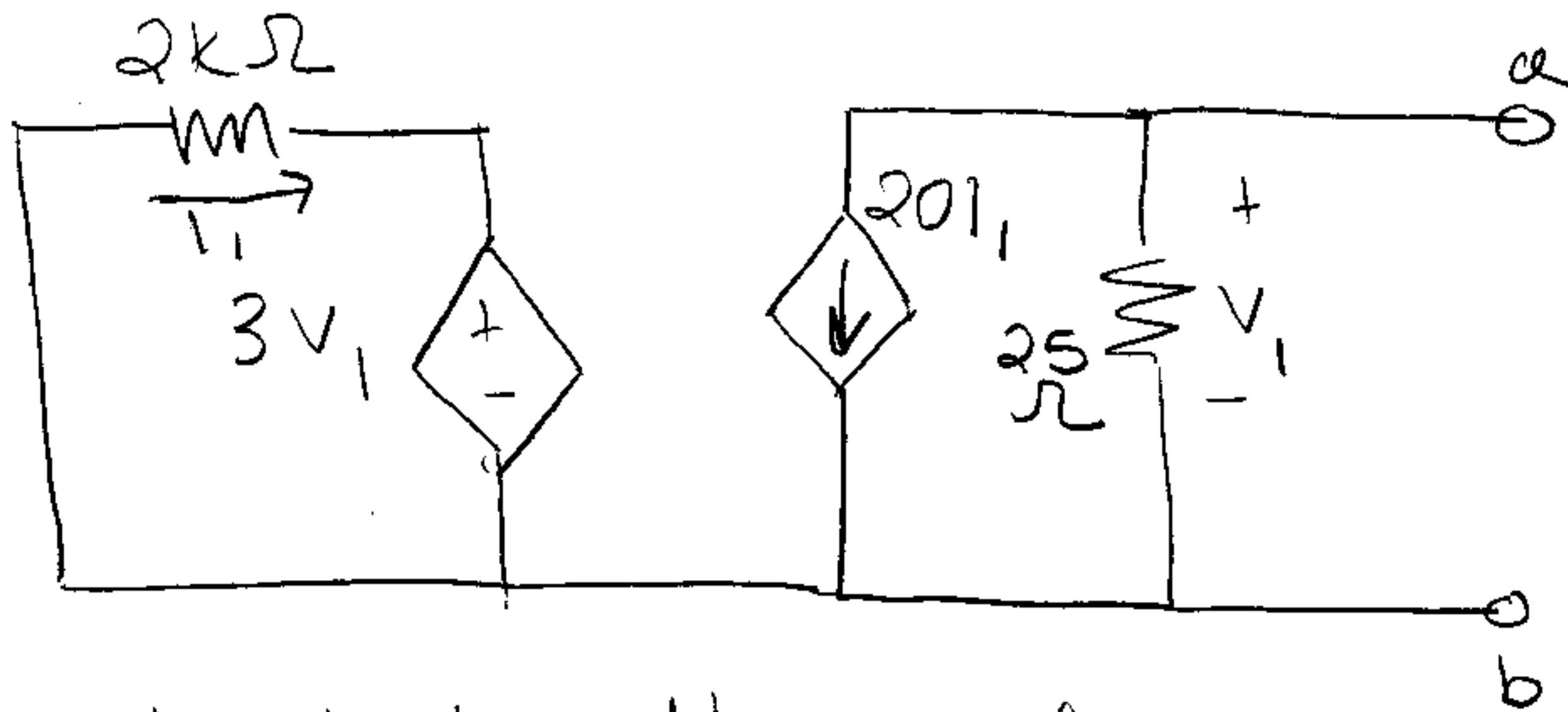
Apply test voltage of 1V.
