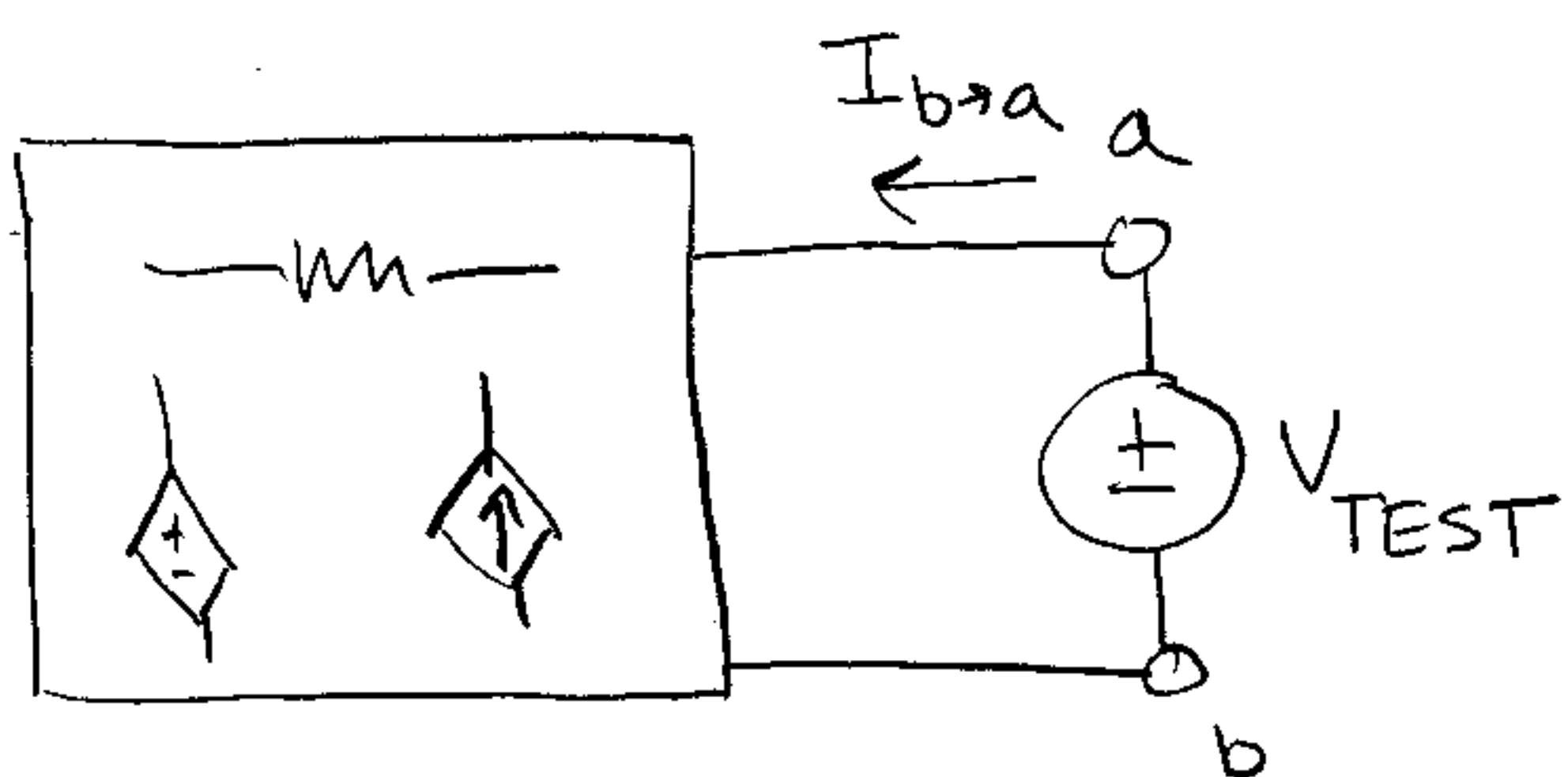
Apply a "test" voltage, measure  $I_{b>a}$ .
