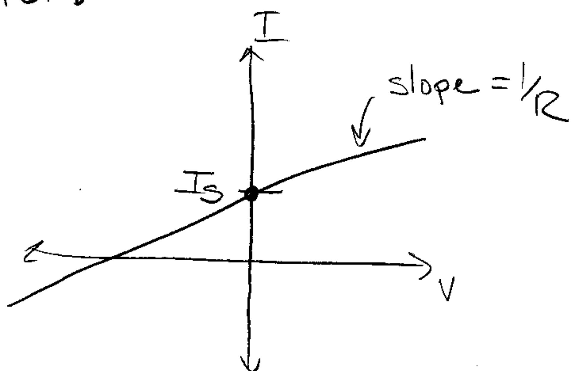
We can also replicate any\* linear circuit through choice of  $I_S$  and  $R$ .
