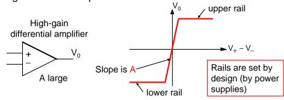
If  $V_+ > V_-$ , the output Vo will be at the upper rail. If  $V_+ < V_-$ , the output Vo will be at the lower rail.
