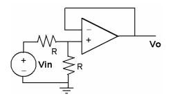
Vo is Vin/2 **regardless** of what is attached to output.
