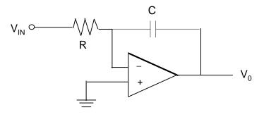
$$V_{o}(t) = -\frac{1}{RC} \int_{0}^{t} V_{IN}(T) dT + V_{C}(0)$$
