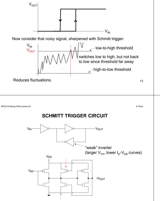
middle transistors have higher threshold magnitude, shallower  $I_D$  vs  $V_{DS}$  curves
