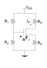
$V_{GS} = V_{DD} \frac{R_2}{R_1 + R_2} - I_D R_S$
