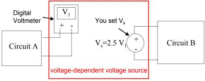
Note that the red box has two wires in (to read the input voltage) and two wires out (to deliver the output voltage).
