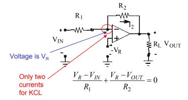
$$V_{OUT} = V_R - \frac{R_2}{R_1} \left( V_{in} - V_R \right)$$
