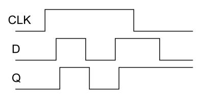
When CLK is high, latch is transparent, when clk is low, latch
