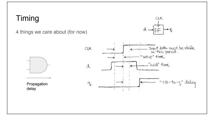
Combination logic propagation delay (max) - after this, the output stably represents the function applied to the input
