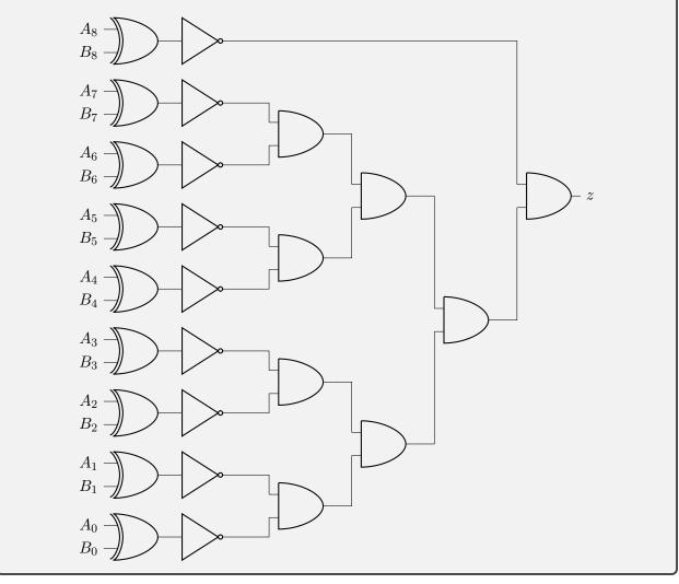
There is a way to do it with one fewer level. First, think about the naive implementation but with ORs, to isolate the use of the inverter. Then observe that this inverter, which you will inevitably use, can be put in a path parallel with the OR tree (or part thereof). You can then use the multiplexer to select the output of the operation on a subset of the bits, based on the input from the operation on a different set. Something like this:
