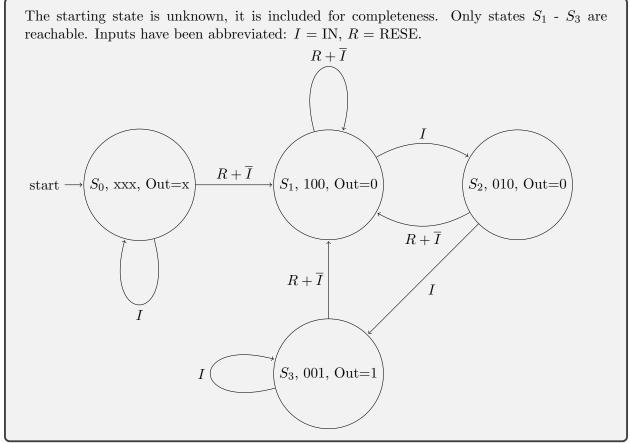
**Optional:** What is the maximum *clock frequency* for this circuit? Assume IN comes from the OUT of an identical copy of this circuit, all logic gates have a delay of 1ns and the flip-flop setup time and clock-to-q delay are both 0.5ns.
