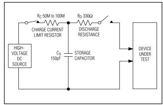
Figure 6a. IEC 1000-4-2 ESD Test Model
