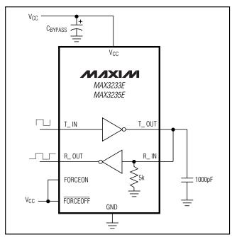
Figure 8. Loopback Test Circuit
