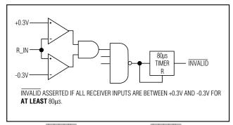
Figure 2a. INVALID Functional Diagram, INVALID Low
