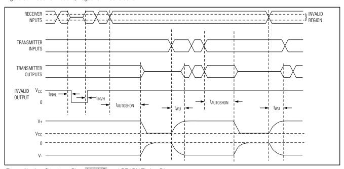
Figure 3b. AutoShutdown Plus, INVALID, and READY Timing Diagram
