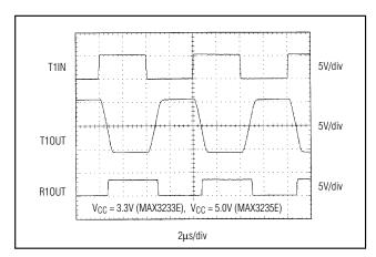
Figure 10. Loopback Test Result at 250kbps
