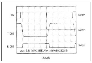
Figure 9. Loopback Test Result at 120kbps
