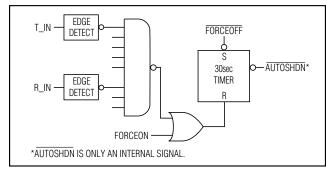
Figure 2c. AutoShutdown Plus Logic
