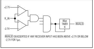
Figure 2b. INVALID Functional Diagram, INVALID High
