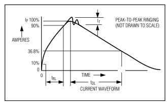
Figure 5b. Human Body Current Waveform
