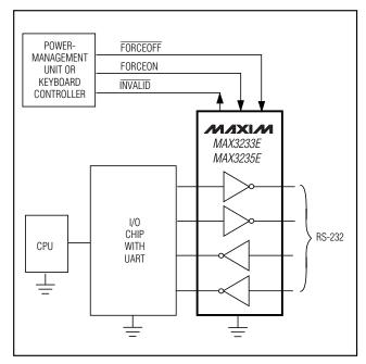
Figure 1. Interface Under Control of PMU
