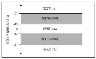
Figure 3a. Receiver Positive/Negative Thresholds for INVALID
