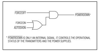
Figure 2d. Power-Down Logic
