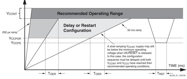
Figure 14: Platform Flash PROM Power-Up Requirements
