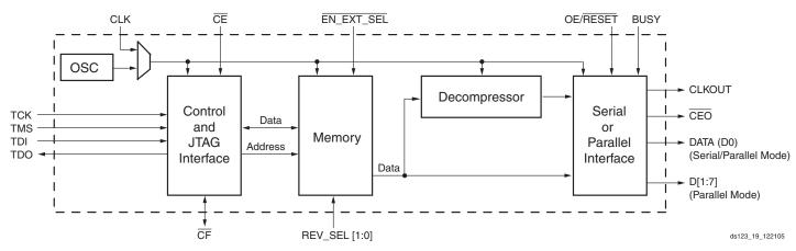
Figure 2: XCFxxP Platform Flash PROM Block Diagram
