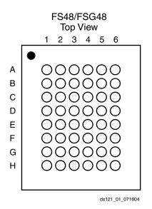
Figure 17: FS48/FSG48 Pinout Diagram (Top View)
