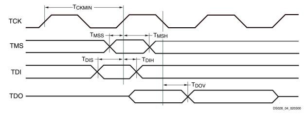
Figure 4: Test Access Port Timing
