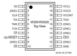
Figure 15: VO20/VOG20 Pinout Diagram (Top View) with Pin Names
