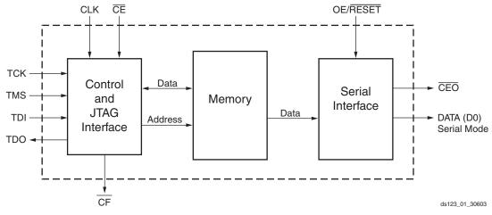
Figure 1: XCFxxS Platform Flash PROM Block Diagram
