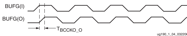
Figure 1-4: BUFG Timing Diagram
