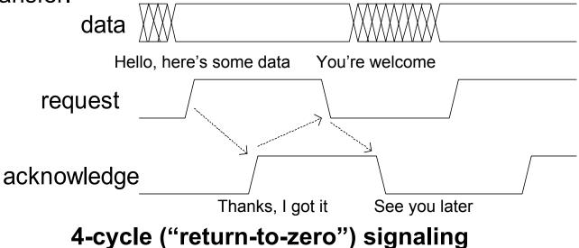
• Note, transfer is insensitive to any delay in sending and receiving.
