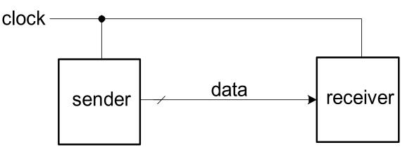
• By design, the clock period is sufficiently long to accommodate wire delay and time to get the data into the receiver.
