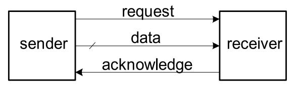
Request/acknowledge "handshake" signal pair used to coordinate data transfer.
