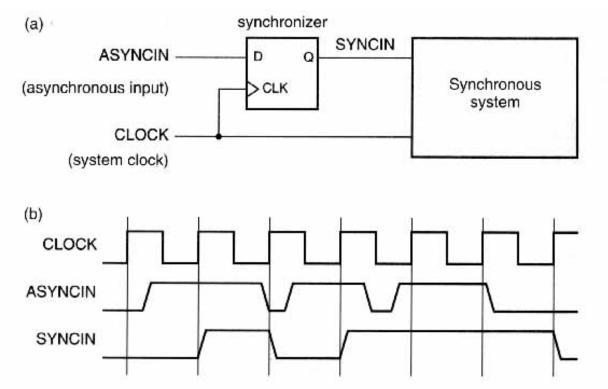
• The D flip-flop samples the asynchronous input at each cycle and produces a synchronous output that meets the setup time of the next stage.
