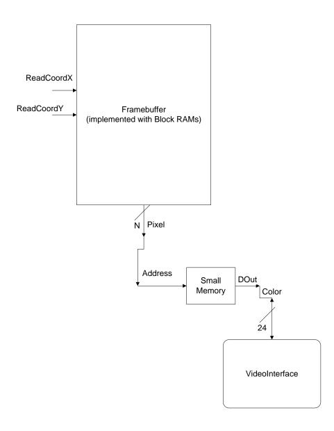
The small memory is 32x24 bit. It has 32 24-bit color entries. This table turns a 5-bit color code into a 24-bit color. Thus, at one time we can display up to 32 out of the  $2^{24}$  displayable colors.
