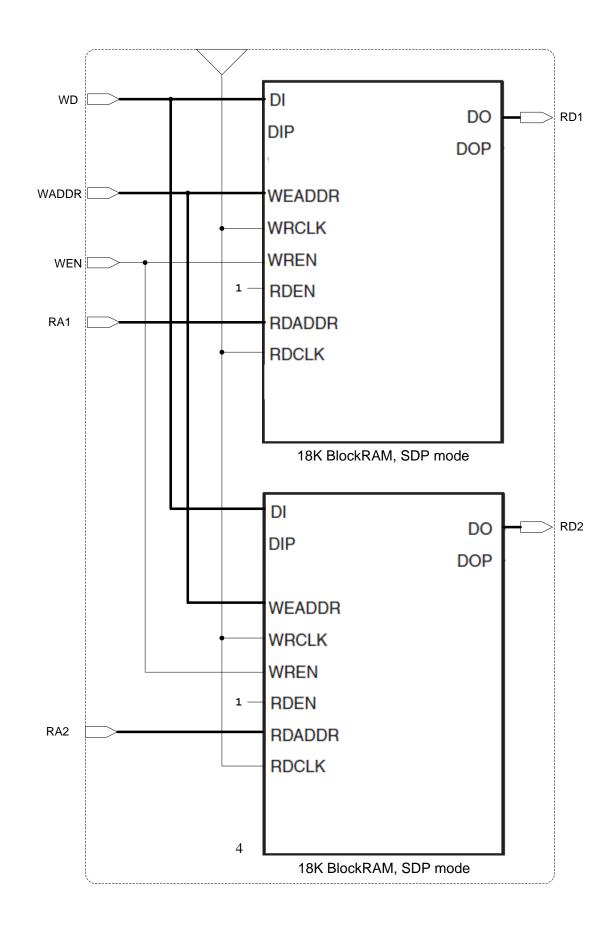
To get a data width of 32, we can use a 18Kb BlockRAM in simple dual-port mode, which allows up to 36 bit data width and independent read and write. We need 2 reads and 1 write on every cycle, so we need to replicate the BlockRAM memory to gain an extra read port. The write port for both RAMs will use the same signals. Using BlockRAMs for a 32x32 regfile wastes most rows in the memory.
