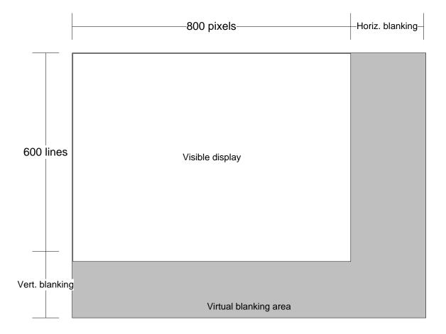
We know the pixel frequency from (c) and just multiply this by the horizontal blanking interval to get how many pixels.
