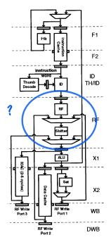
Must consider all connected register pairs, paths from input to register, register to output. Don't forget the controller.
