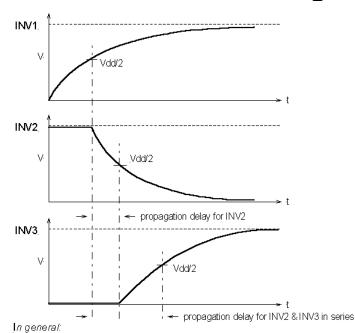
prop. delay = sum of individual prop. delays of gates in series.
