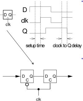
Setup time results from delay through *first* latch.
