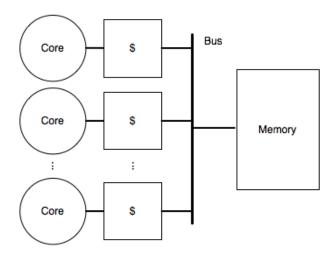
Assume we have many elements (long input vector) for the histogram, and the input data is uniform random. The caches are big enough to hold all the bin data of the histogram. The characteristics of the cache are the same as Q2.C. To keep the caches coherent, we implement a snoopy cache coherence protocol on the bus. We can snoop, invalidate, and transfer the data all in 1 bus access of 10 cycles.
