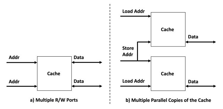
(1) [5 pts] One option to support higher cache bandwidth is to add more ports to the cache, as shown in (a). Alternatively, we could instead maintain multiple parallel copies of the cache as shown in (b). Describe the tradeoffs between supporting higher cache bandwidth through these approaches.
