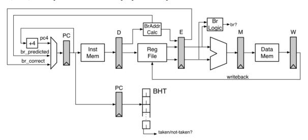
The BHT has been added in the Decode Stage. The BHT is indexed by the PC register in the Decode Stage. Branch address calculation has been moved to the Decode Stage. This allows the processor to redirect the PC if the BHT predicts "Taken".
