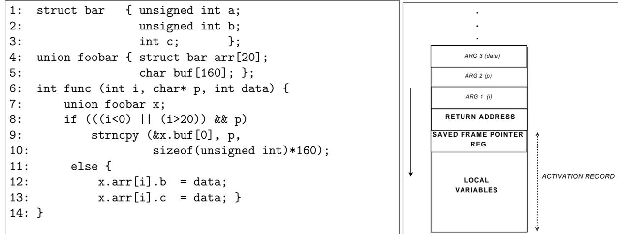
Figure 1: (Left) Vulnerable code (Right) Stack frame layout for function `func`
