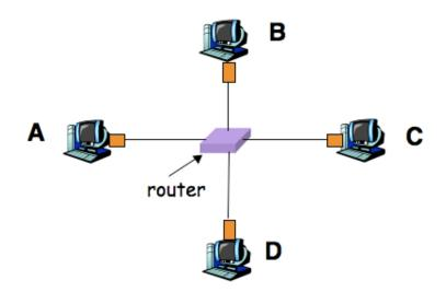
The router functions as follows. When it receives a packet from one of the nodes, the router by default will *broadcast* the packet to all of the other nodes. However, any time a node *sends* traffic to the router, the router *remembers* the link that connects to that node, so in the future for any packet sent *to* the node, the router can send the packet directly, rather than broadcasting it.
