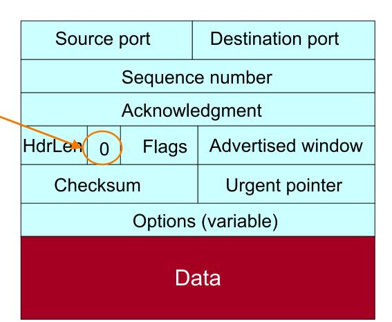
Buffer space available for receiving data. Used for TCP's sliding window.
