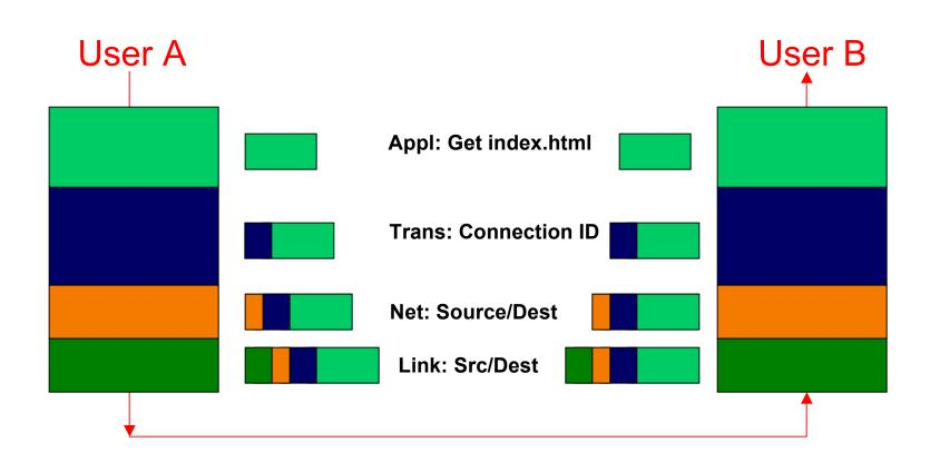
Common case: 20 bytes TCP header + 20 bytes IP header + 14 bytes Ethernet header = *54 bytes overhead*
