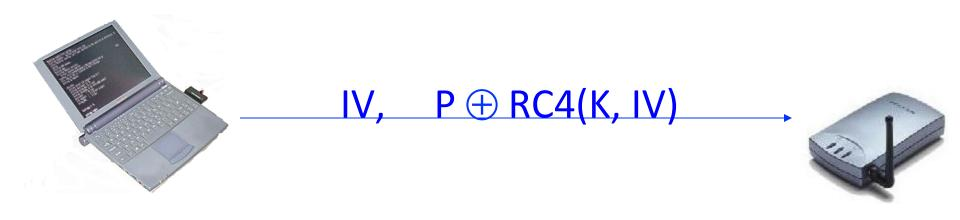
WEP uses the RC4 stream cipher to encrypt a TCP/IP packet (P) by xor-ing it with keystream (RC4(K, IV))
