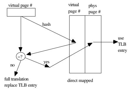
As a (bad, as we will see shortly) example, could use the lower bits of virtual page number to index TLB. Compare against the upper bits of virtual page number to check for match.
