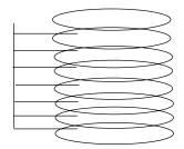
Disk is read via a comb – 2 read/write "head assembly" at end of each arm (typically, only put disk heads to read inside surfaces, external surfaces are too exposed).
