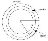
Disk **surface**: circular disk, coated with magnetic material Quarter-sized to 12 - 14" platters
