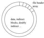
UNIX refers to file by index into array - tells it where to find the file header
