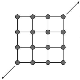
This structure will not resist shearing
