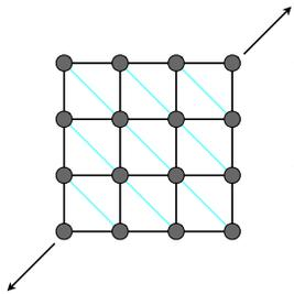
This structure will resist shearing but has anisotropic bias
