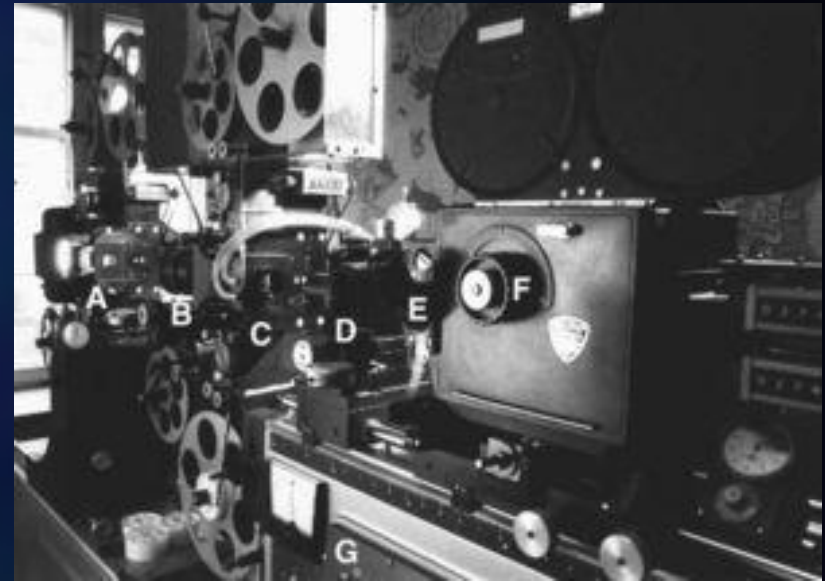
An optical printer used for optical effects
