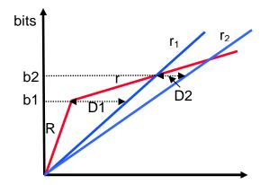
If r2 > r1 then the total queueing delay is D1 + D2 and the (see figure above). In particular, we have D1 + D2 = b1\*(R-r1)/(R\*r1) + b2\*(R-r2)/(R\*r2), where b2 = b1\*r1\*(R-r)/(R\*(r1-r)).
